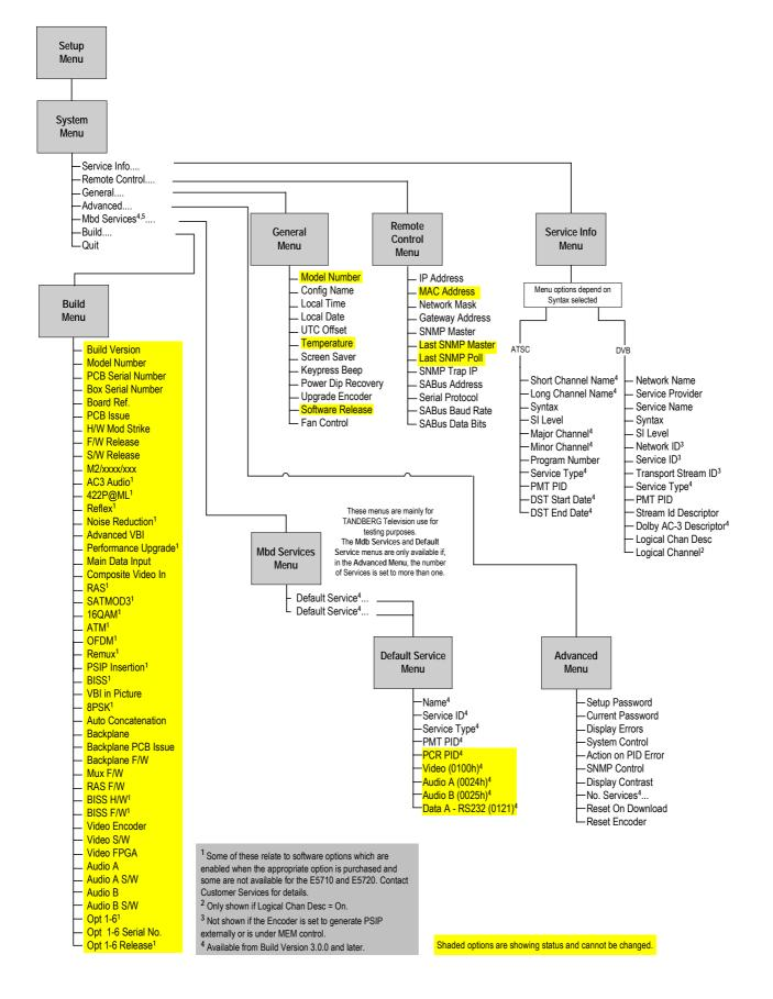
Figure 4.9: Menu Hierarchy – Setup/System Menu
